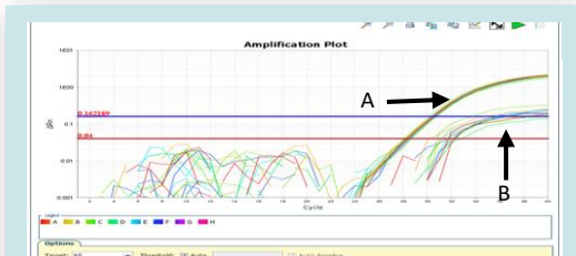
Figure 1. A: Arrow shows logarithmic expression of IC B: Arrow shows unspecific amplification.
